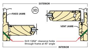
E. Drill a 13/64" clearance hole through the door frame at each indentation in the extrusion at the top (head) of the door frame.
